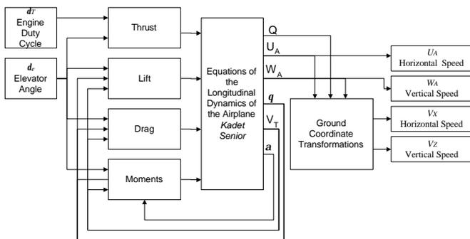
Figure 2: Block diagram of the mathematical model.
