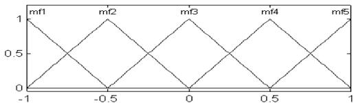
Figure 8: Membership functions for the acceleration.
