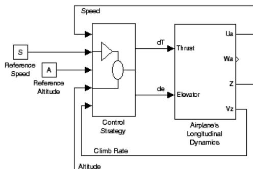
Figure 3: Basic control diagram used for the three strategies.
