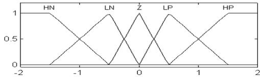
Figure 14: Membership functions for the climb rate.
