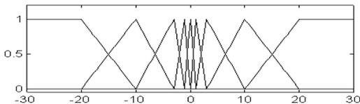
Figure 7: Membership functions for the speed error.
