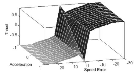
Figure 9: Surface formed by the output of the fuzzy controller for the speed.
