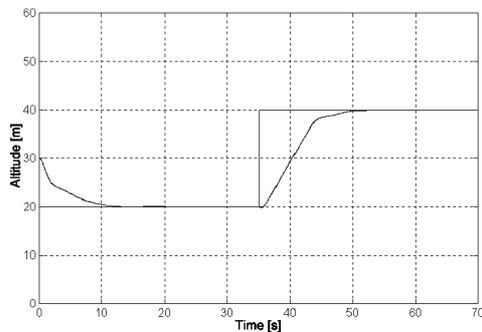
Figure 20: Hybrid control of altitude.
