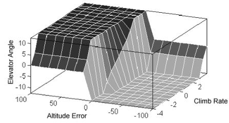
Figure 12: Surface formed by the output of the fuzzy controller for the altitude.
