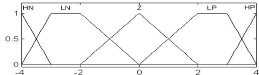
Figure 10: Membership functions for the climb rate.
