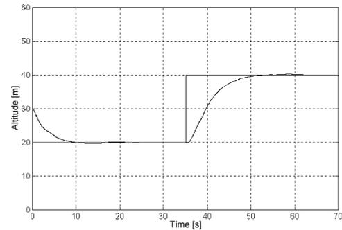
Figure 16: PID control of altitude.
