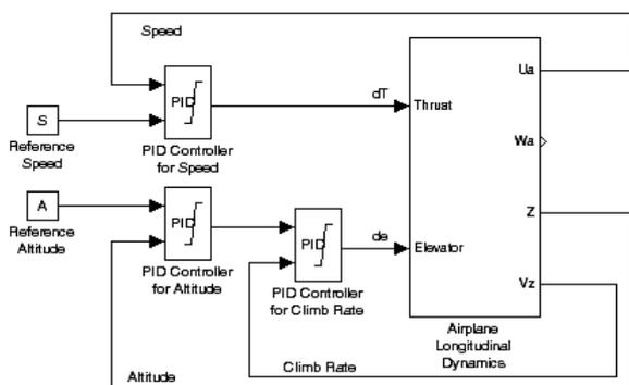
Figure 4: Block diagram of the PID controller system.
