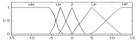
Figure 11: Membership functions for the altitude error.
