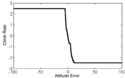
Figure 15: Output-input function for the altitude fuzzy controller.
