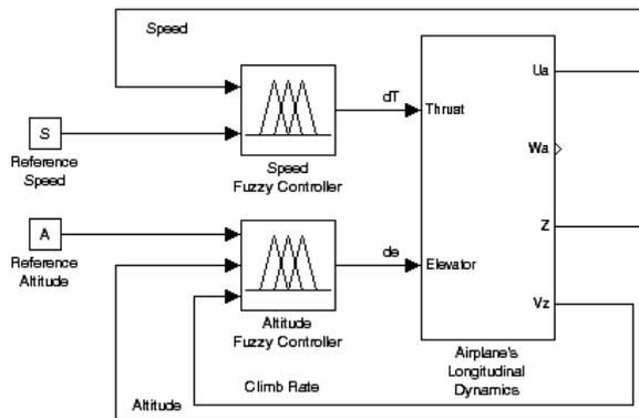
Figure 5: Block diagram of the fuzzy control system.
