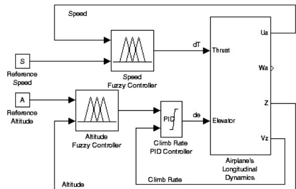
Figure 13: Block diagram of the hybrid controller system.
