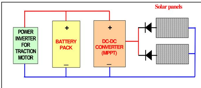
Fig.3. Electric diagram of the solar EV
