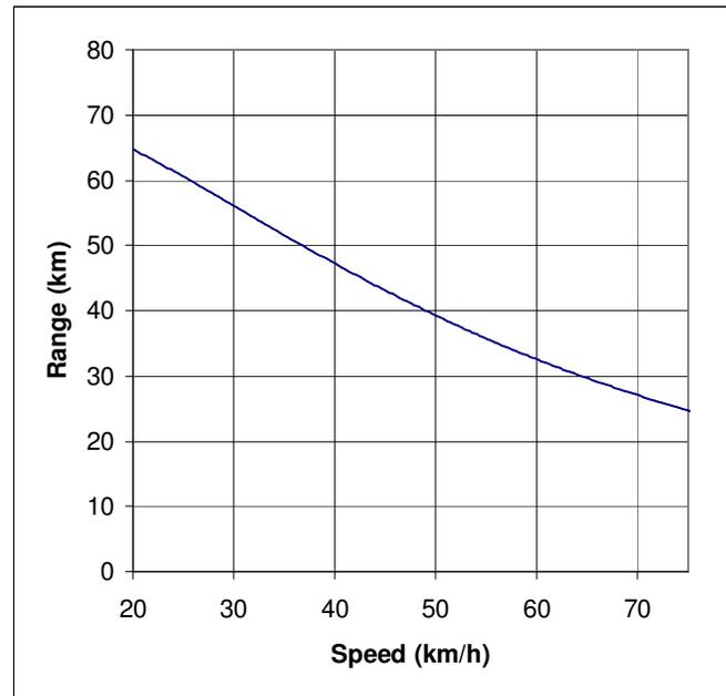
Fig.1. Range as a function of speed in a small EV
