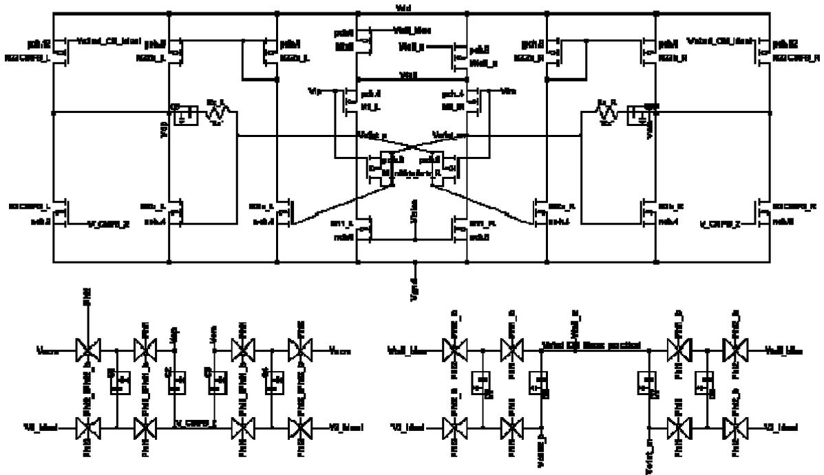
Figure 8. Integrator OTA schematic.
