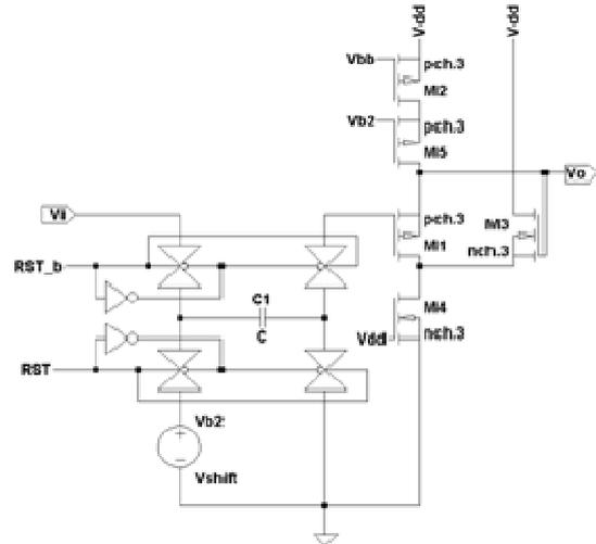
Figure 6. Simplified buffer schematic.
