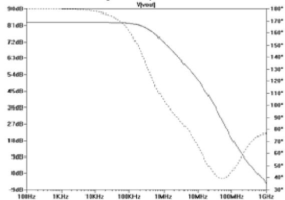
Figure 9. CSA frequency response in magnitude (solid line) and phase (dashed line).
