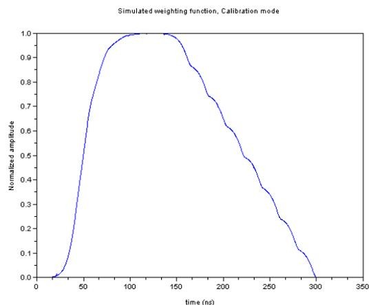
**Figure 11. Simulated weighting function for calibration mode.**
