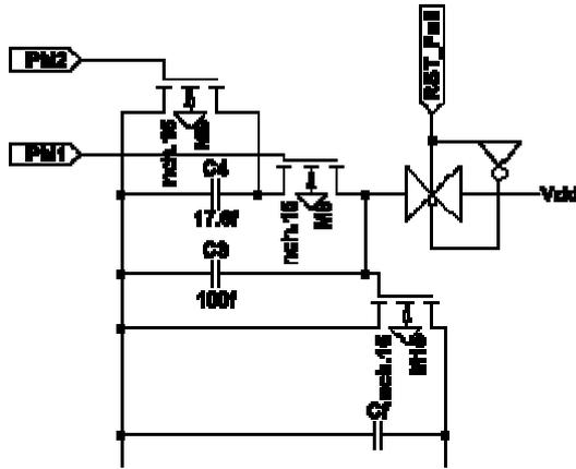
Figure 5. CSA reset circuitry.
