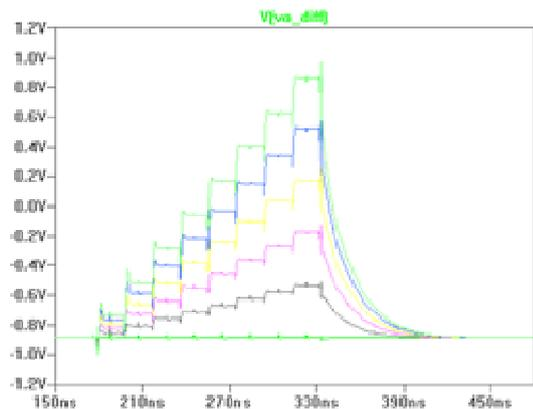
**Figure 10. Front-end output waveforms for calibration operation.**
