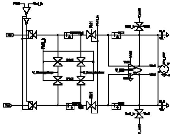
Figure 7. Switched-capacitor integrator schematic.
