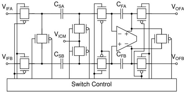
Fig. 5. Simplified schematic of the filter.
