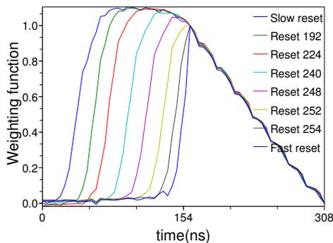
Fig. 19. The Bean prototype measured weighting functions for different reset schemes, DCal mode.
