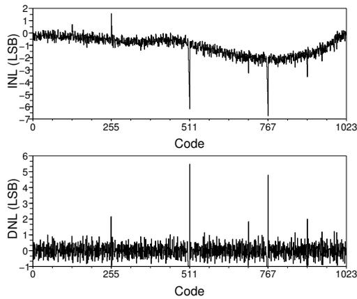
Fig. 16. The Bean prototype linearity test results, SDT mode.
