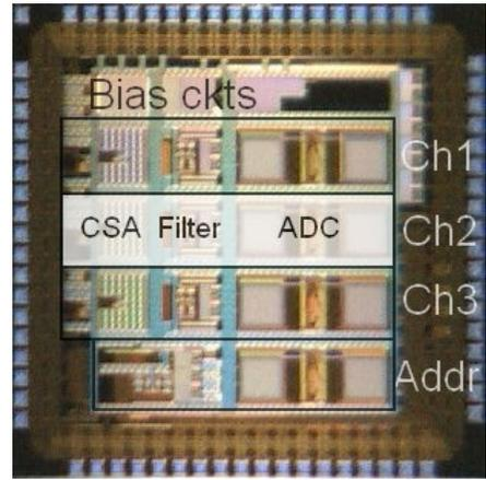
Fig. 13. Microphotography of the Bean prototype.
