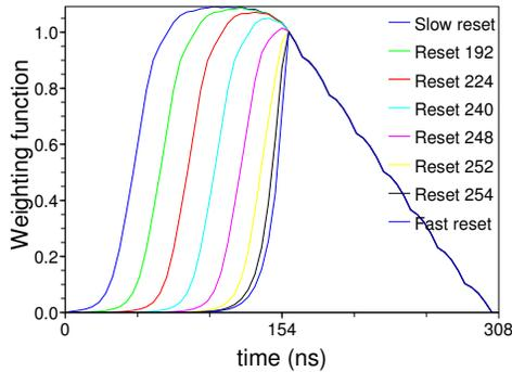
Fig. 18. The Bean prototype simulated weighting functions for different reset schemes, DCal mode.
