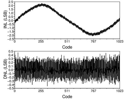
Fig. 14. MOM capacitor ADC linearity test results.
