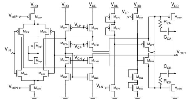
Fig. 11. Rail-to-rail buffer schematic.
