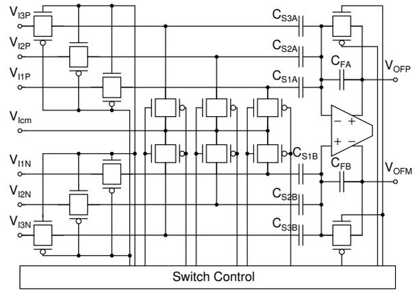
Fig. 9. Adder schematic.
