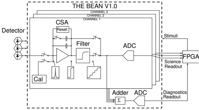
Fig. 2. The Bean prototype simplified block diagram.
