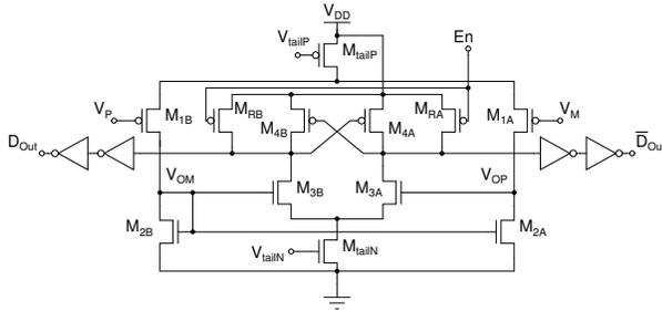
Fig. 8. ADC comparator schematic.
