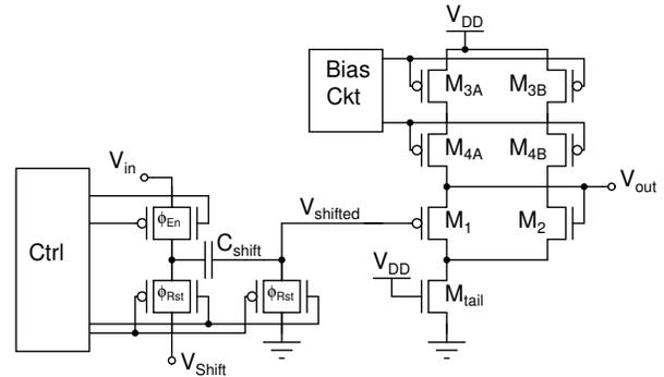
Fig. 10. Signal buffer schematic.
