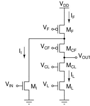
Fig. 3. Schematic of CSA amplifier. Bias circuits have been omitted.
