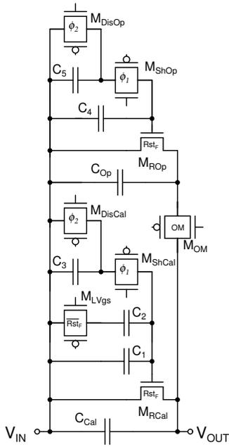
Fig. 4. Schematic of CSA feedback network.
