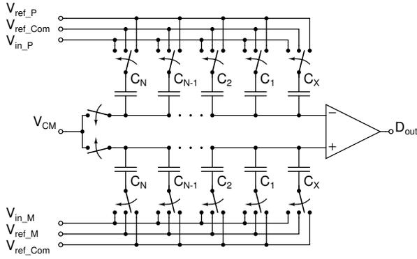
Fig. 7. Simplified schematic of the SAR ADC. The logic circuits have been omitted.
