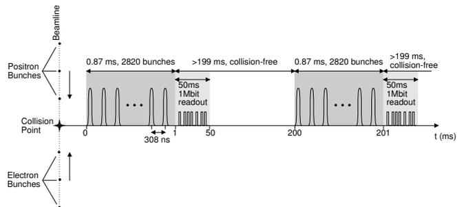
Fig. 1. Structure of the ILC pulse train.
