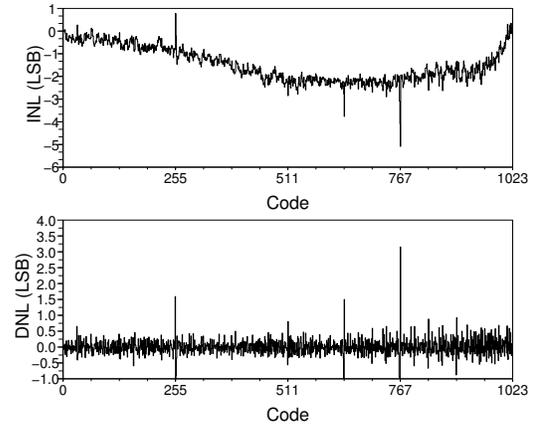
Fig. 17. The Bean prototype linearity test results, DCal mode.
