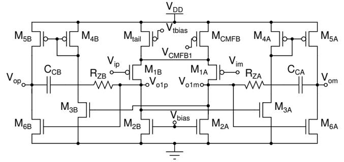
Fig. 6. Simplified schematic of the filter OTA. The common-mode feedback networks have been omitted.
