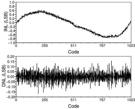
Fig. 15. MIM capacitor ADC linearity test results.
