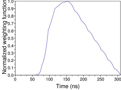
Fig. 12. Simulated weighting function in the DCAL mode, for a switched-capacitor integrator and slow reset-release technique.
