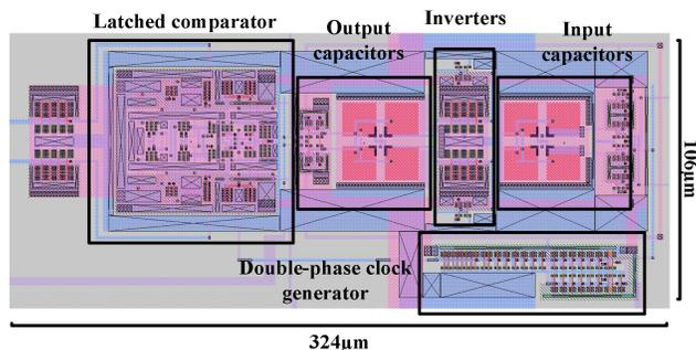
Fig. 4. Fully-differential offset-cancelling circuit and latched comparator layout.
