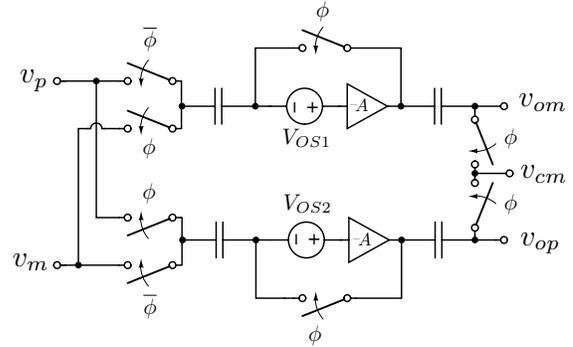
Fig. 1. Fully-Differential offset-cancelling circuit simplified schematic.
