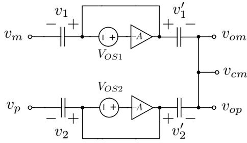
Fig. 2. Equivalent circuit at the first step of operation when the switches controlled by  $\phi$  are closed.
