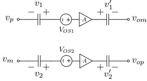
Fig. 3. Equivalent circuit at the second step of operation when the switches controlled by  $\bar{\phi}$  are closed.
